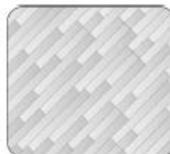
3-board stagger diagonal
